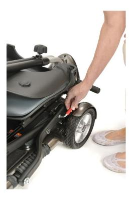
2. Pull the tiller away from the floor pan until the front wheels of your Minimo touch the floor.
