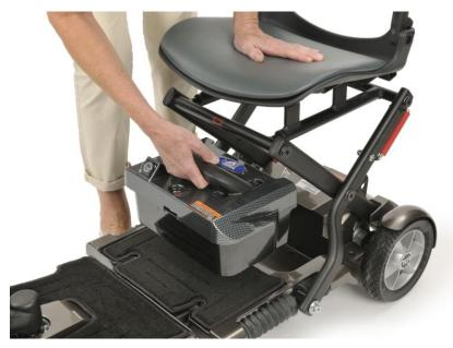
To remove the battery pack of your Minimo first ensure the pack is unlocked by inserting the key into the pack and turning it 90° anti clockwise to the unlock position. Then simply lift the pack up away from the base of the scooter and the seat using the handle provided.
