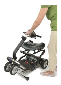
3. Ensure your Minimo is locked in the unfolded position by pulling the chair away from the floor pan with one hand and pushing the tiller away from the seat with the other until you hear a click and feel you Minimo lock into this position. Once your Minimo is locked in position you will no longer be able to move the tiller towards and away from the seat so use this as a simple test to find out if you Minimo is locked in the unfolded position.
