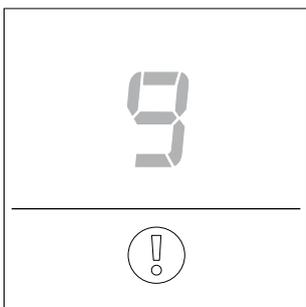
If the remote control does not detect the two wheels (for example, due to a poor remote communication), the information message shown here appears on the display.
