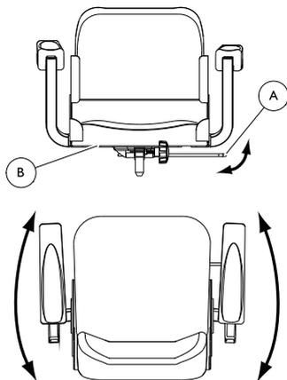
1. Pull up the seat lock lever **A** to unlock the seat **B**.
