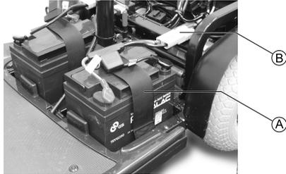
3. Secure the batteries to the base frame using the battery retention strap (A). Securely tighten.
