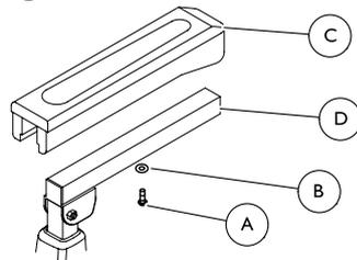
1. Remove the mounting screw **A** and washer **B** that secure the armrest pad **C** to the armrest **D**.
