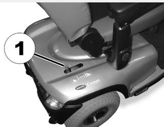
The lever for engaging and disengaging the motor is located on the right-hand side at the rear.
