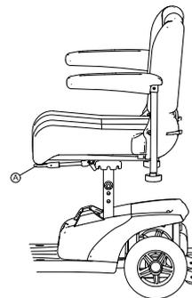
Lift the detent lever **A** up.
