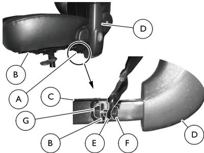
1. Locate the mounting bracket **A** below the seat **B** on the seat frame **C** near the armrest **D**.
