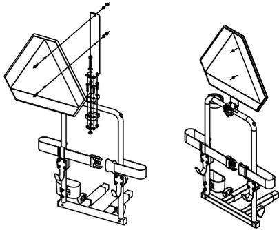
I. Position the rear reflector as shown in the drawing.
