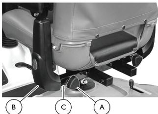
1. Loosen the knob **A** securing the armrest tube **B** to the seat frame **C**.
